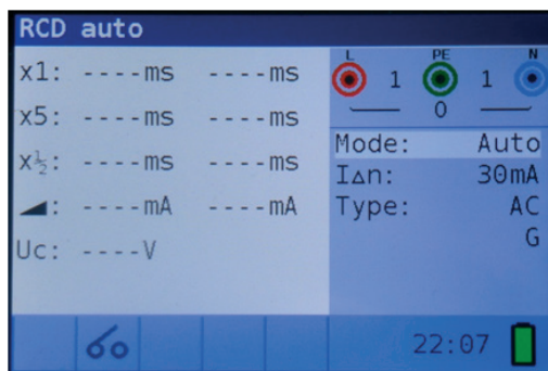
Figure 4 18: RCD autotest menu
